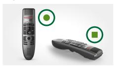
Being on the cutting edge of technology, the SpeechMike Premium Air comes with an integrated motion sensor, meaning it can be controlled by the movement of your hand. It detects when it's put on the table, mutes the microphone, and once it is being picked up again it unmutes the microphone. In addition to that, custom events can be programmed, e.g., to pause and to continue the recording.
