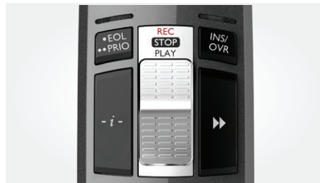
Slide-switch operation (record, stop, play, fast rewind)
